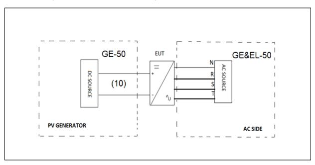
Different equipment has been used to take measures as it shown in chapter 2.4. Current and voltage clamps have been connected to the inverter input / output for all the tests.
